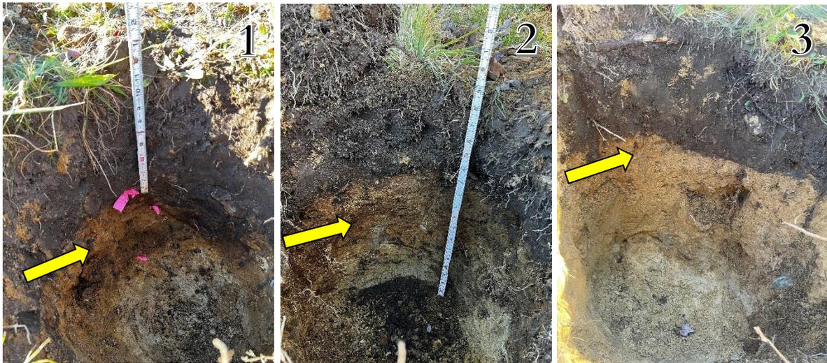
**Photographs 1-3** View of BVW 1 test pits from left to right: Test Pit #1, Test Pit #2, Test Pit #3. View of dark yellowish brown colors (yellow arrows) indicative of upland soils directly beneath the Ap horizon.
