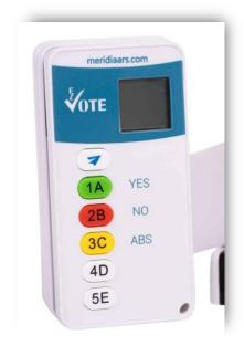
The signals are securely transmitted to a central computer that automatically calculates vote margins for a simple, 2/3, or any other majority. The computer can be connected to a projector to display the results after the voting period has closed.
