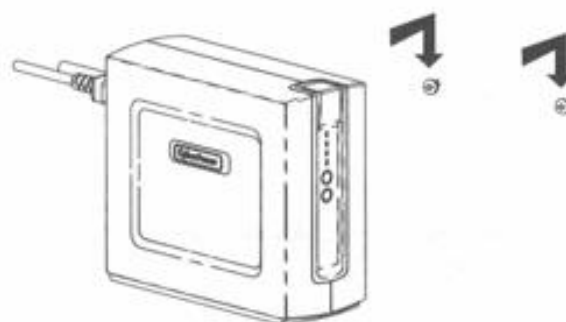
Step 4: Use the enclosed wall mount template to locate screws on the wall. Hang the DTC36U12V on the screws which are located on the wall.
